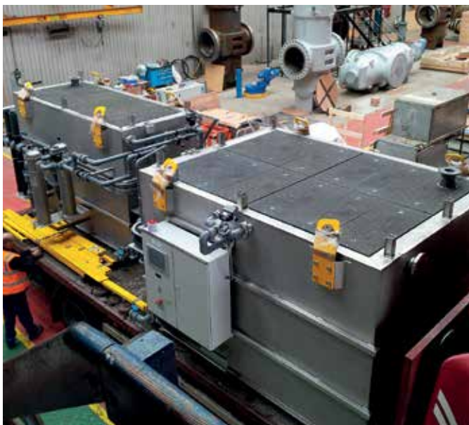
The two systems were adapted for Fibrelite trench covers for access from above
