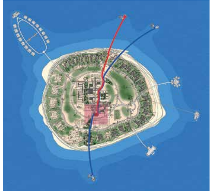
Island overview with fuel delivery jetty (red) fuel storage (box in centre) and refuelling jetty (blue)
